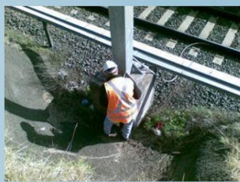
Impact-echo investigation to determine pile depths of overhead structures
