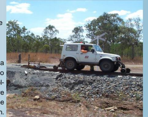
A hi-rail vehicle towing the trolley with GPR antennae. The data logging system is located within the vehicle allowing for safe and efficient operation.
