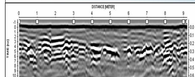
Timber girder profile containing a termite pipe / void along its length.
